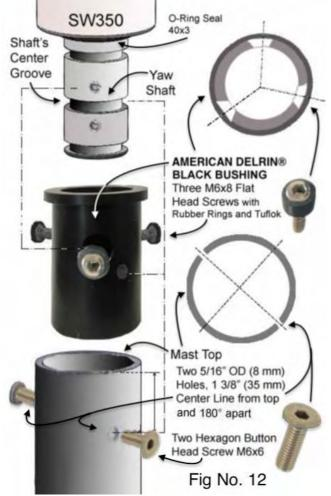
screws (with TUFLOK applied to the threads) are used to attach the bushing to the mast. These screws extend into the groove of the yaw shaft, but will not touch it (see Fig. No. 7).
