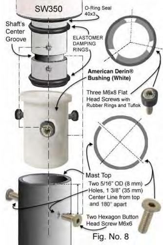
attaching the bushing to the SW350's yaw shaft and to the mast. Three (3) M6 x 8 Socket cap screws with TUFLOK coated threads and rubber rings (Fig No. 8) are used to attach the bushing to the yaw shaft. Two (2) M6 x 6 hexagon socket button head screws are used to attach the bushing to the mast. (Optional M6 x 12 hexagon socket button head screws are also included). These screws will extend into the groove of the yaw shaft, but should not touch it.
