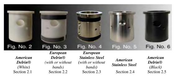
Bushing selection depends on the type of location the turbine will be deployed in. American and European Delrin<sup>®</sup> bushings are used for integration on ships and other salt water applications. American and European Stainless Steel bushing are used on tall towers and in locations subject to higher wind speeds, as well as Mobile platforms (such as trailers).
