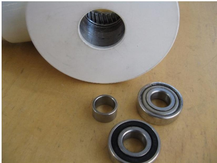
**Technician note: Installation of the new bearing must be done while the generator housing is still hot. Otherwise, the generator will need to be reheated to 80°C/176 deg F.**
