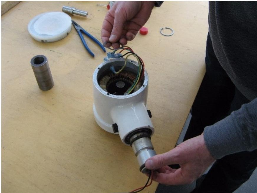
6. Install the snap-ring into the bore of the bearing.
