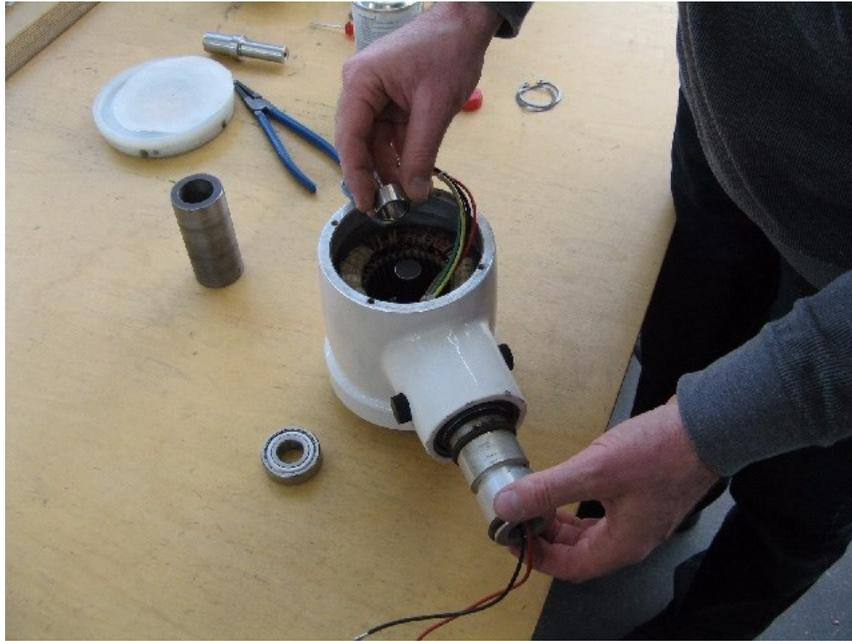
3. Insert the rear bearing and press slightly.
