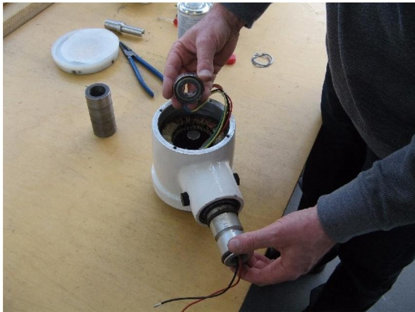
4. Use the PVC pipe to press the bearing in.
