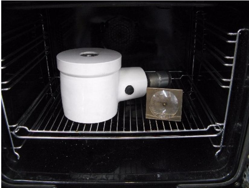
6. Once the generator has reached temperature, remove the generator from the furnace and place on a suitable work surface. Remove the two roller bearings and the spacer bushing; push slightly if required to remove.
