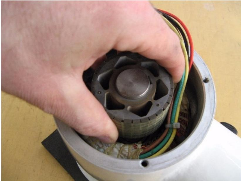
The rotor in position after proper installation.
